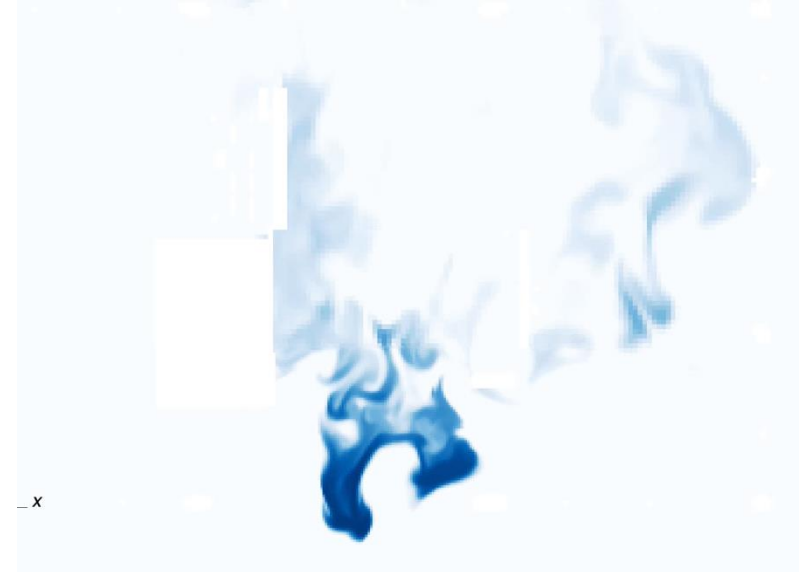
Vertical slice in first level of Mobile Launcher colored by mass fraction of water
