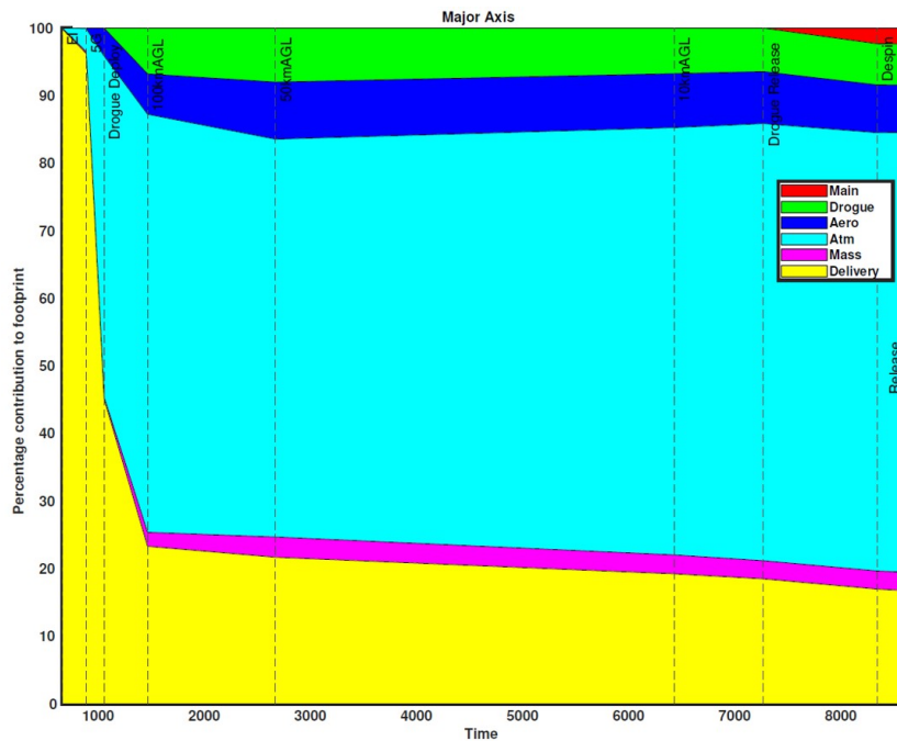
Fig. 19 The sensitivity of the major axis of the lander separation footprint with respect to the dispersions
