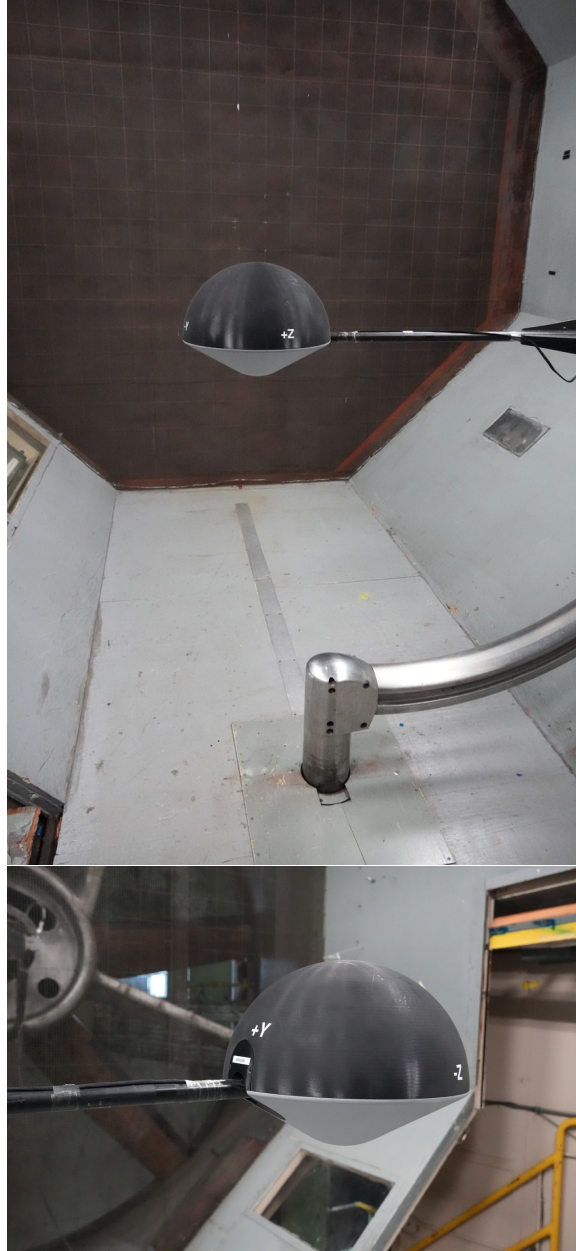
Fig. 1 NASA's 12-foot Low-Speed Tunnel with sting mount and test article setup.
