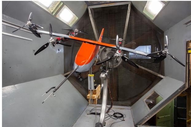
**Fig. 11 RAVEN-SWFT vehicle mounted on a 3DOF free motion wind-tunnel apparatus.**
