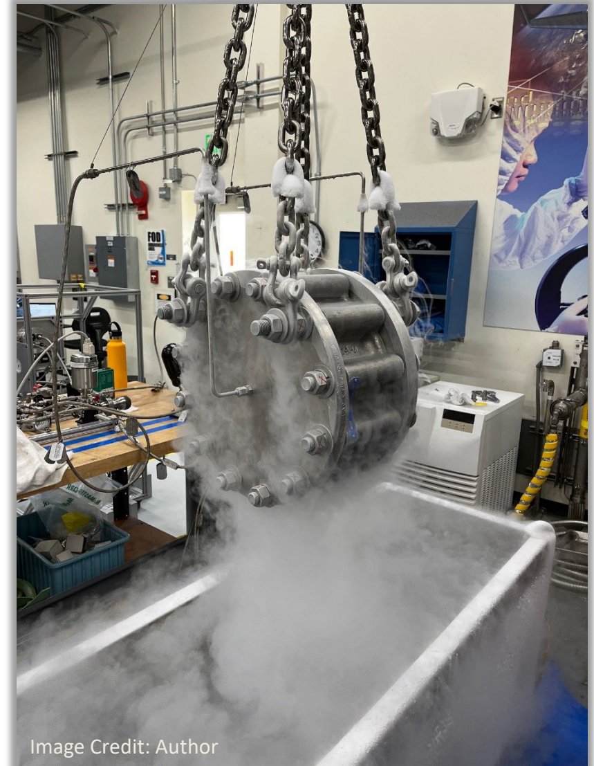
10” Check Valve Acceptance Test at the Cryogenics Test Laboratory
