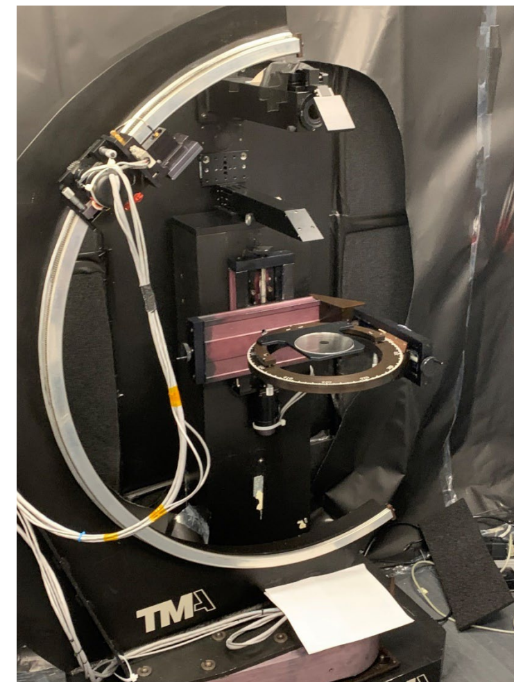
Goniometer, Angle of incidence zenith and azimuth, Scatter angles zenith and azimuth, Sample positioning in X-Y-Z directions and rotation.
