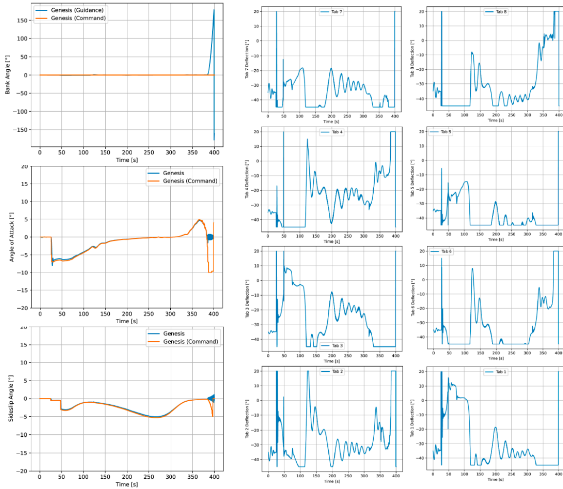
Figure 12: Wind Angles and Flap Deflection Responses for Baseline Target Values (Target Final: Mach 2.1)
