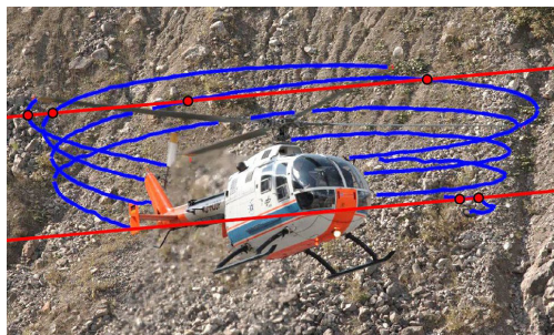
Fig. 16 Multi-camera mapping of helicopter vortices in hover using natural background BOS and epipolar analysis [142]. Image used with permission of the authors.
