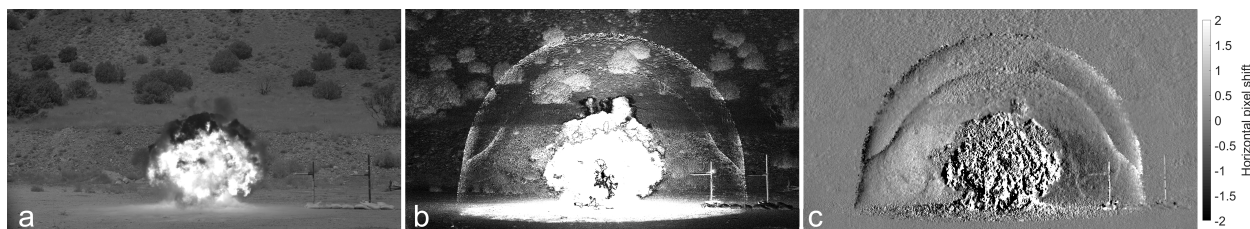
Fig. 15 (a) A high-speed image of a 1 kg C-4 explosion is compared to a pre-test image and processed with (b) pixel intensity subtractions or (c) optical flow algorithms to visualize the shock wave produced. Images used with permission of the authors.
