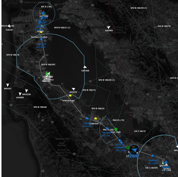
Fig. 1. Example of the Tactical Situation Display used for the UAM Communications Modality Experiment. Cyan airspace boundaries (Class B/C airspace – solid, Class D airspace – dashed) highlight those that are co-altitude with the UAM flights. Checkpoint locations for radio calls are designated with yellow flags [12].
