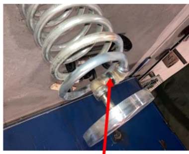
(a) : 90-degree elbows were added at each end of the helical tube component
