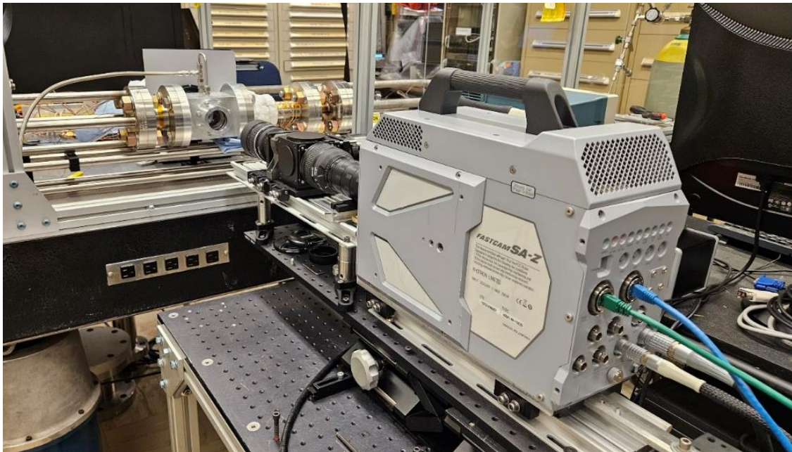
Figure 24. SAFS System Looking Through the Optical Spool Piece Installed on the TAHP
