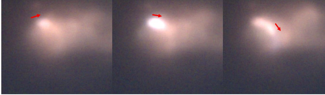
Fig 8. Images of test 002 clockwise rotating detonation from high-speed video.
