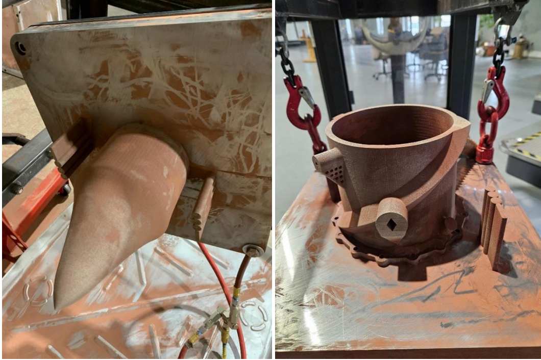
Fig 3. Kerosene RDRE GRCop-42 inner body (left) and outer body calorimeter nozzle extension (right) during the depowdering process.
