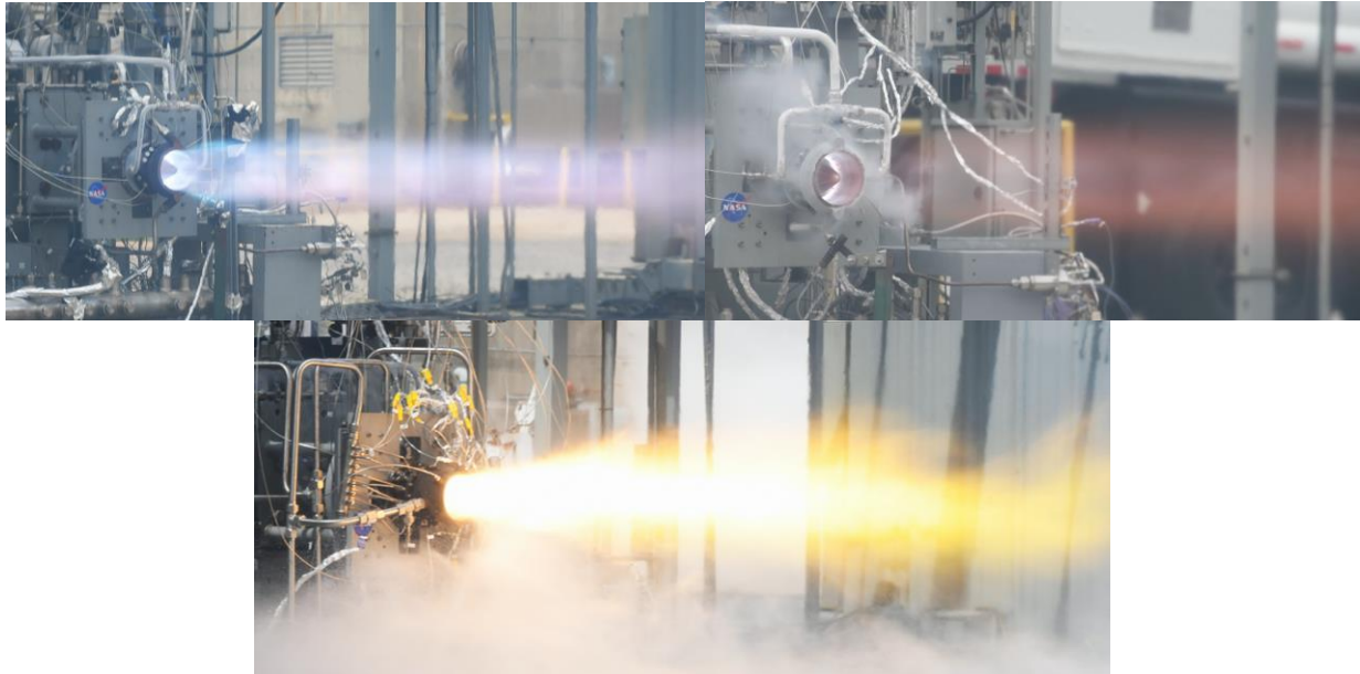
Fig 1. NASA RDRE pivotal hot fire tests using methane/oxygen (top left), hydrogen/oxygen (top right), and RP1/oxygen (bottom).
