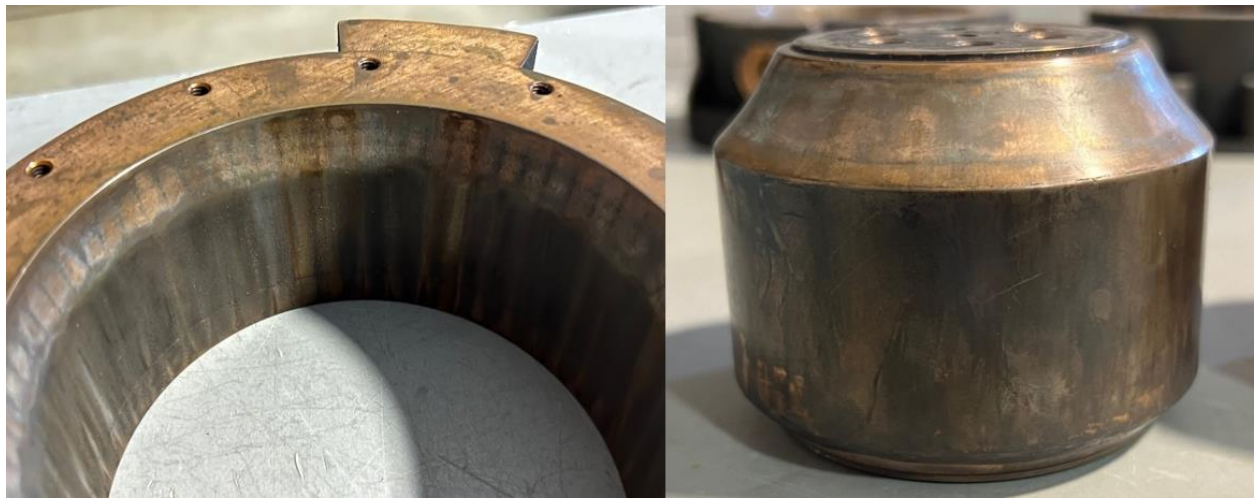
Fig 11. Purdue/NASA CIF hardware post dozens of hot fire tests courtesy of Dr. Ariana Martinez from [13].
