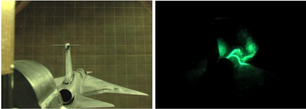
Fig. 14 Aircraft model being tested with and without flow visualization in the 12-Foot Low-Speed Tunnel. The photo on right shows forebody vortices being visualized by the smoke wand/laser light sheet system. (Credit: NASA)
