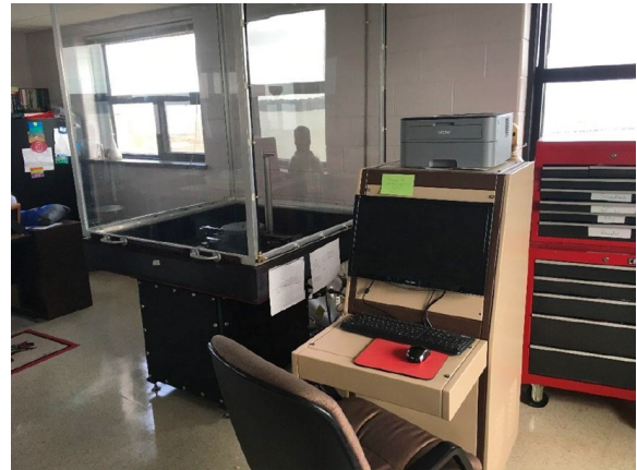
Fig. 16 CG/MOI measurement instrument for dynamically scaled models. (Credit: NASA)
