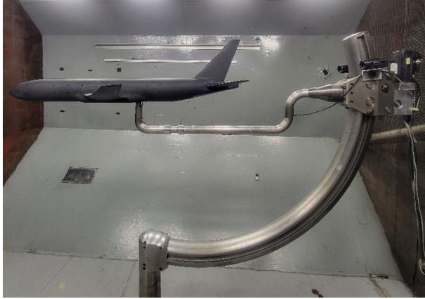
Fig. 17 Model mounted on the C-strut in the 12-Foot Low-Speed Tunnel. (Credit: NASA)
