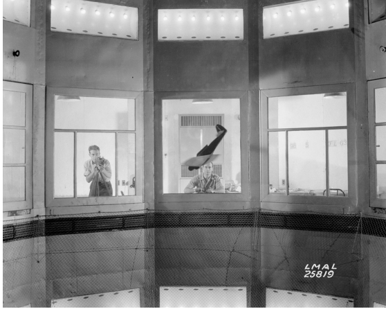
Fig. 5 Model under test in the 20-Foot Vertical Spin Tunnel in 1941, shortly after the VST became operational. (Credit: NASA)
