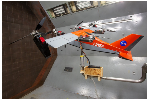
Fig. 24 Vehicle mounted on the 3-DOF rig in the 12-Foot Low-Speed Tunnel. (Credit: NASA)
