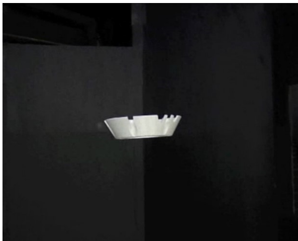
Fig. 37 FBC conducting free-flight test after jettison from the CM. (Credit: NASA)
