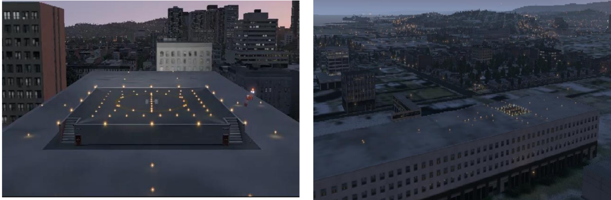
Figure 9. Vertiport Design and Simulation. Showing simulated landing light pattern design at the vertiport (left) and approach light pattern along the building top (right).
