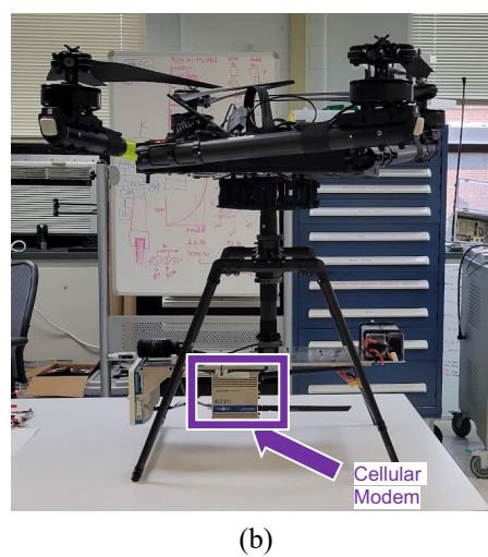
Figure 9: Onboard Payload as seen from port (a) and starboard (b) sides with research payload annotated.
