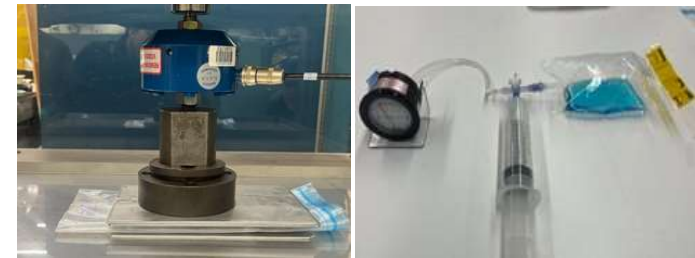
Figure 2: photos from static load test and functional leak testing of FEP bags. Freezer test will be conducted at JSC cold stowage group.
