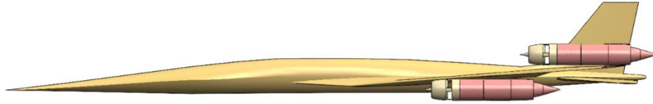
Fig. 3 Under-wing engine STCA variant used for PUR Technical Challenge.
