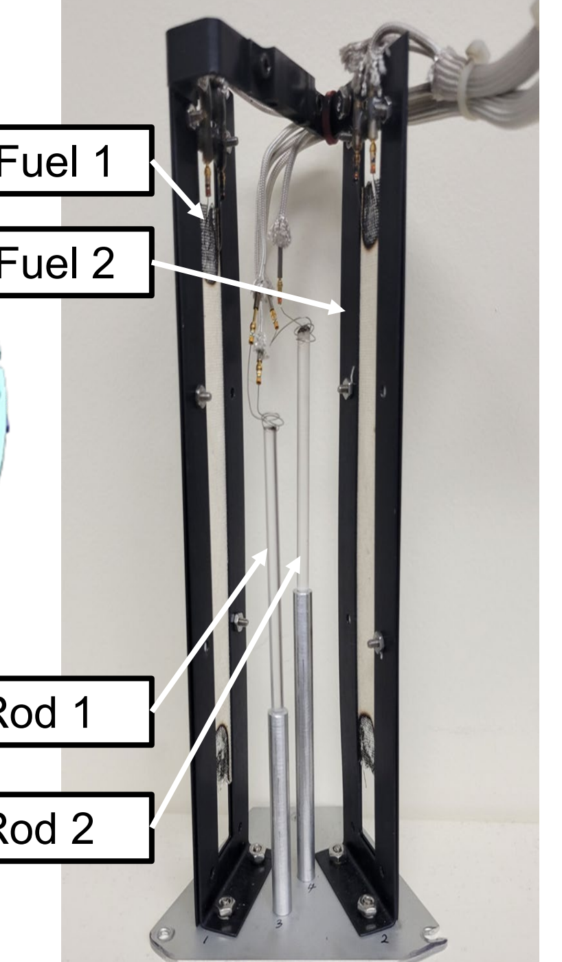
Flammability of Materials on the Moon (FM 2 ) Solid Fuel Module
