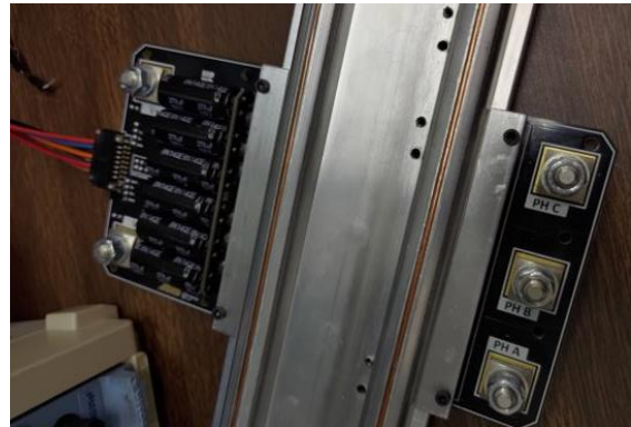
Figure 5: Electronic speed controller setup for QUEEN V1 testing. ESC was cooled using a cold plate mounted directly to the PCB.
