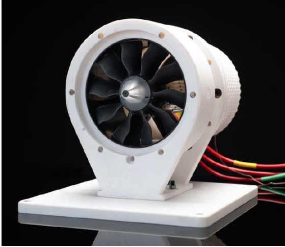
Figure 2: The COTS EDF was installed in the NASA custom-designed 3D printed containment shroud and the aft duct and pedestal mounting plate are visible. The bellmouth and inlet duct acoustic liner sections were not installed in this photograph.
