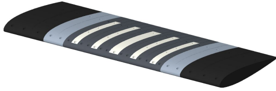
(a) 3-D printed wing sections including fan placement parts (dark gray) and associated plugs (white), spacers (light gray), and wingtips (black).
