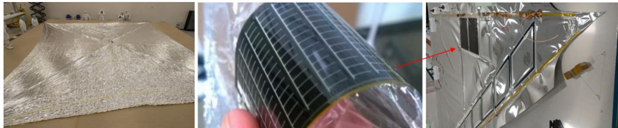
Fig. 2: Substrate and thin-film solar cell assembly that comprise the PowerSail. The NEAScout solar sail deployed (Left). A ‘LISA-T’ Thin-film solar cell stack up (Middle). A ‘LISA-T’ stack up embedded on a solar sail (Right).
