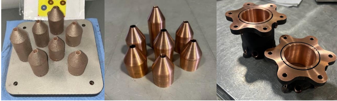
Figure 3. MARLEN inner bodies before HIP (left) and after machining (center) and outer bodies after machining (right).
