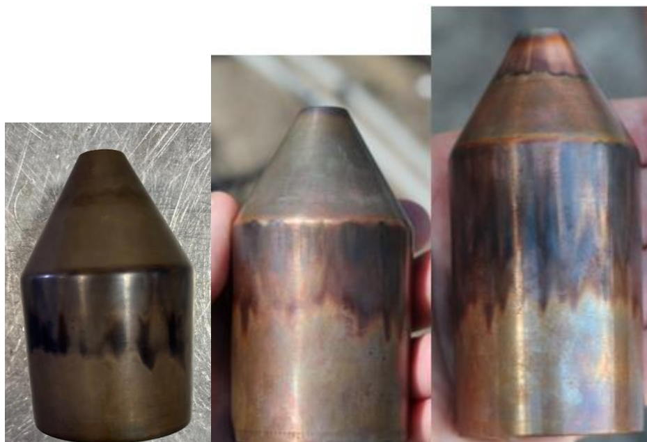
Figure 9. Heat staining on the inner body inside the annulus for the 1.5", 2", and 2.5" L' inner bodies.
