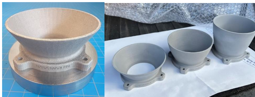
Figure 5. C-103 radiatively cooled nozzles post print (left) and post processed (right).
