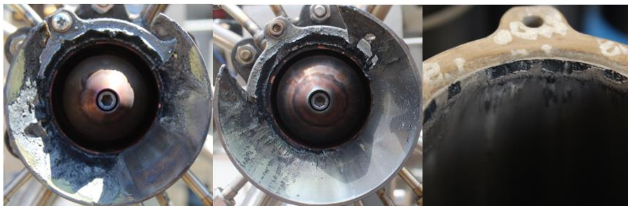
Figure 10. Radiatively cooled nozzle failure modes of 1.4" (left), 2" (center), and 3" (right).
