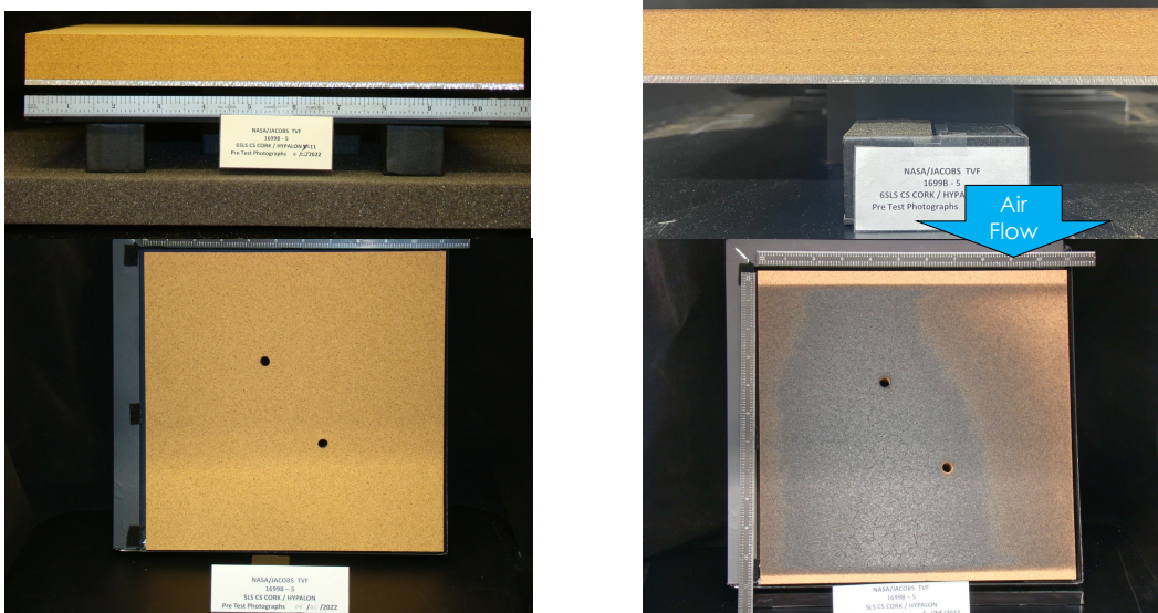
Figure 20. Run 82: (top-left) side and (bottom-left) top-down views of pre-TVC test TPS panel; (top-right) side and (bottom-right) top-down views of post-TVC test TPS panel.
