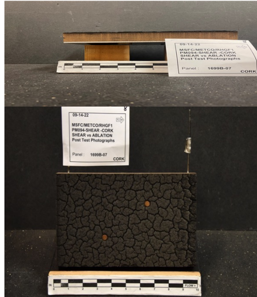
Figure 22. HGF Run 9: Pre-HGF test TPS sample top-down and side images (left) and post-HGF test TPS sample images (right).
