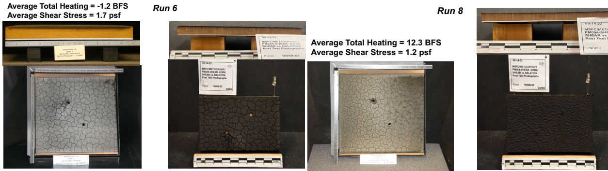
Figure A3. HGF Runs 6 and 8: Pre-HGF test TPS sample top-down and side images (left) and post-HGF test TPS sample images.
