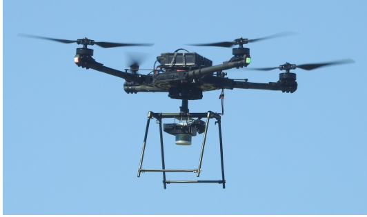
(a) Multicopter drone Alta X, used as tracked vehicle
