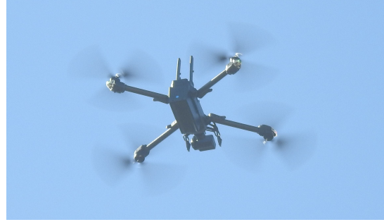
(b) Skydio drone, used as airborne observer
