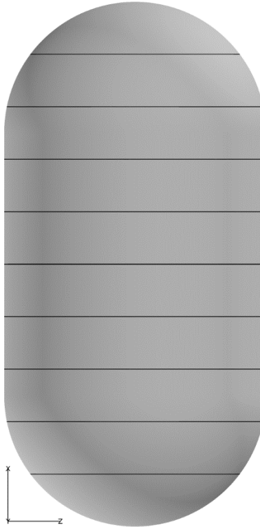
Fig. 6 Analyzed tank geometry with liquid fill levels at 10% by volume increments shown.
