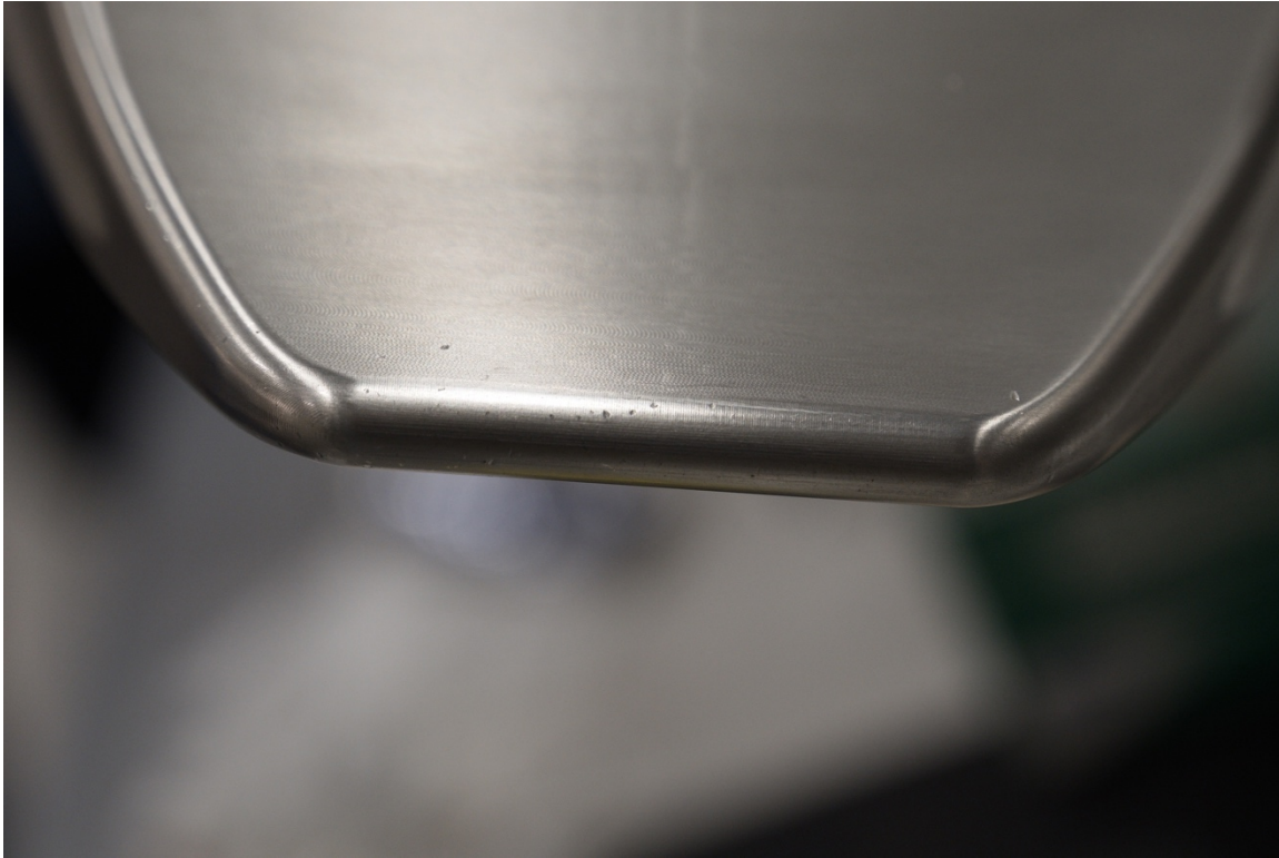
Close up of Side B nose, showing small damage sites [Source: AFRL]
