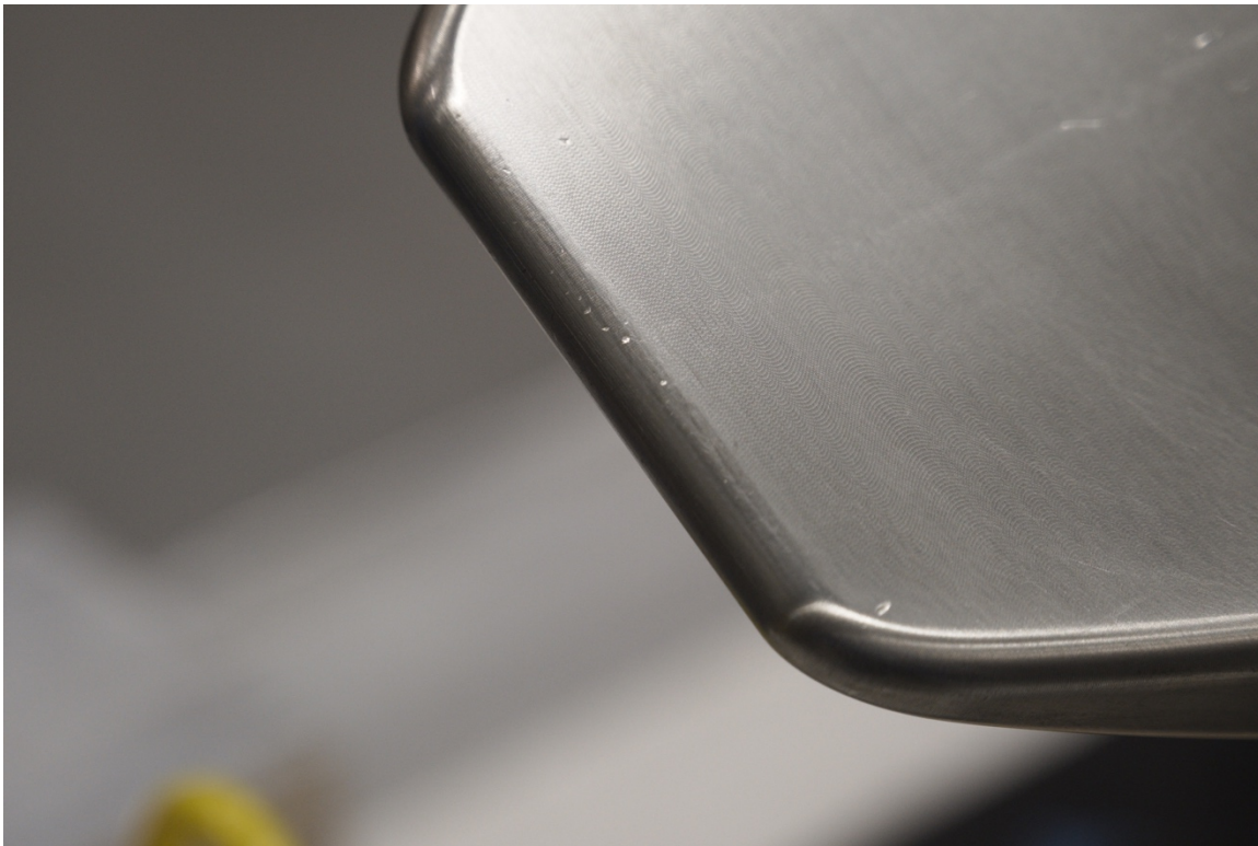
Close up of Side B nose, showing small damage/defect sites [Source: AFRL]
