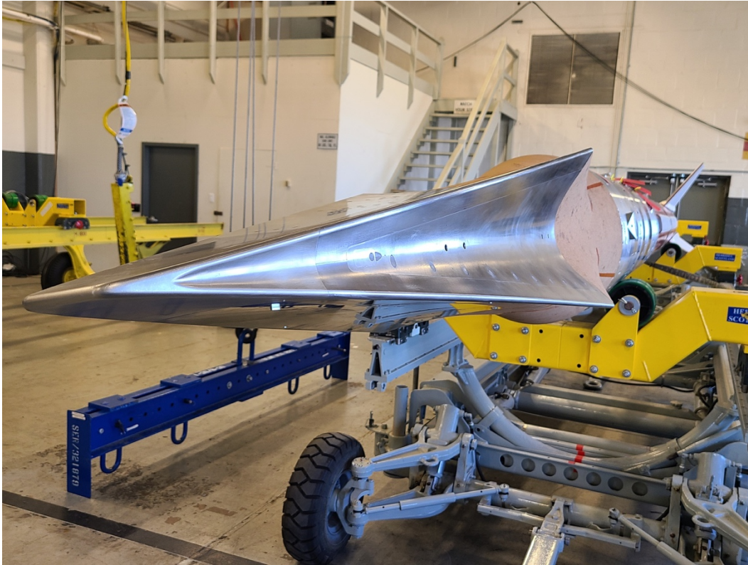
Side view of BOLT-2 showing one of the gutters [Source: AFRL]
