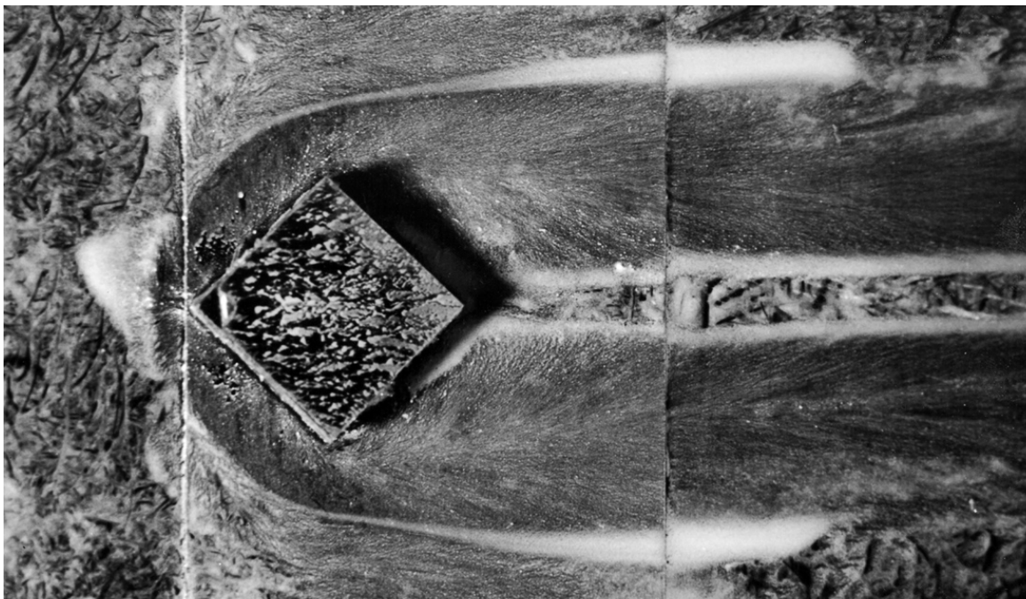
Oil-flow image showing surface streamlines around diamond trip
