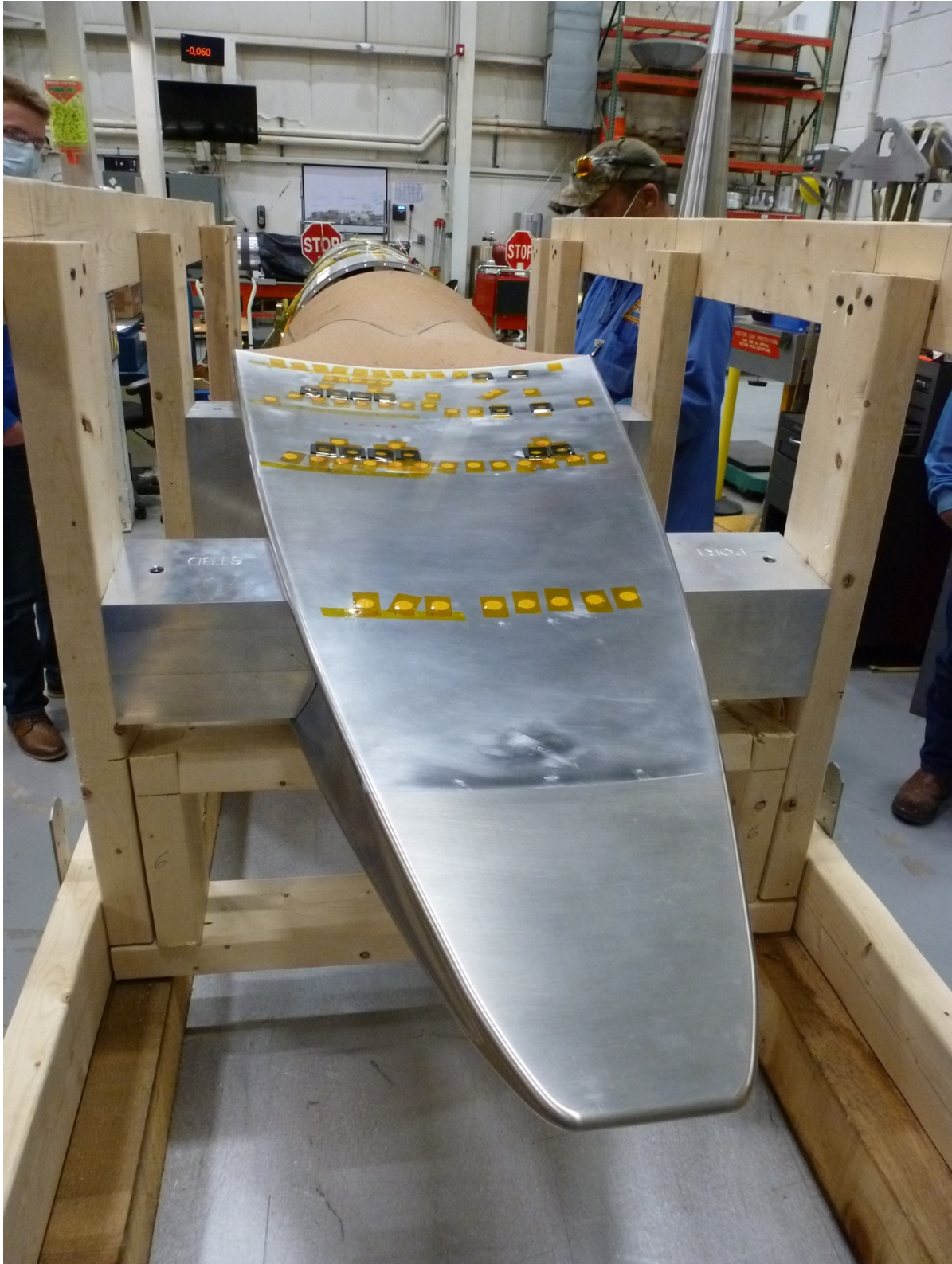
Side A – note handling blocks indicating port & starboard [Source: AFRL] Yellow tape covers various sensors during pre-flight handling
