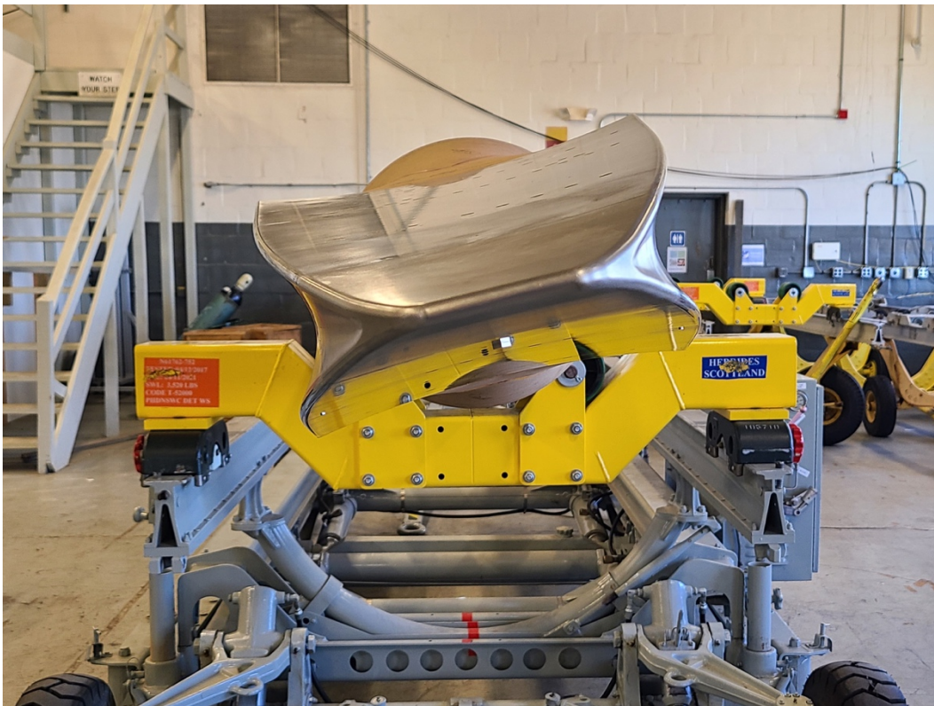
Front view of BOLT-2 showing difference between the two sides [Source: AFRL]
