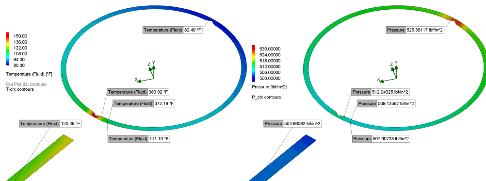
Fig. 6 Coolant pressure drop and bulk/film temperatures from CFD/CHT analysis.
