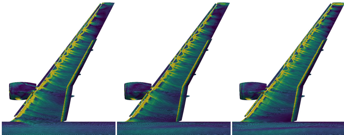
(b) Time-averaged skin friction coefficient magnitude with surface skin friction lines.
