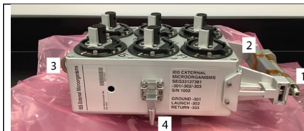
Figure 1: The sampling kit contains eight swab canisters in total (six on the top and two on the bottom). A reusable end effector (1) is used to remove and reinstall the swabs. The kit also contains a handrail (2), tether loop (3), and, bayonet probes(4) to allow easy manipulation during EVA.
