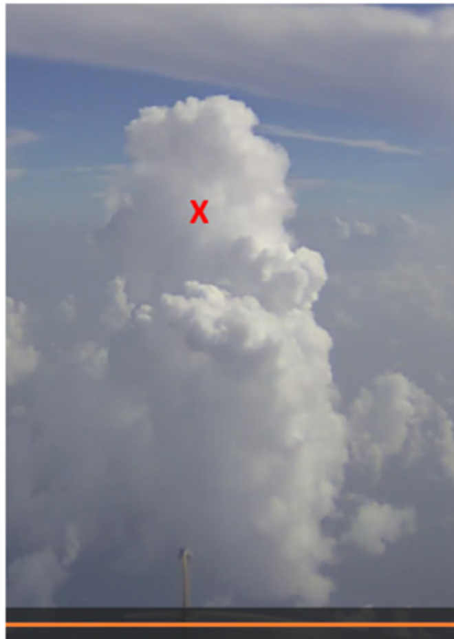
Figure 4.27.—Frame from DC-8 forward video before entry into cloud of 2022-07-26 at 3.8 °C. Red X is approximate location of entry. In-cloud time was 10 s.
