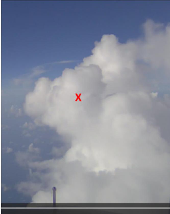
Figure 4.31.—Frame from DC-8 forward video before entry into cloud of 2022-07-26 at approximately -9.8^{\circ}\text{C} . Red X is approximate location of entry. In-cloud time was 16 s.
