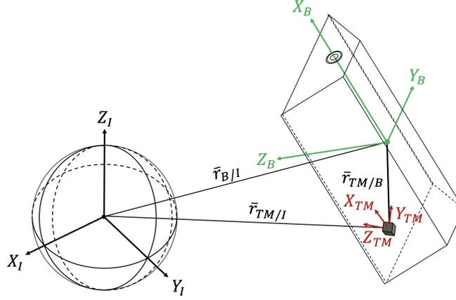
**Figure 2. Frames of Reference. The Inertial Frame ( $I$ ), Body-Fixed Frame ( $B$ ) and Test Mass Frame ( $TM$ ) are illustrated along with their respective position vectors**
