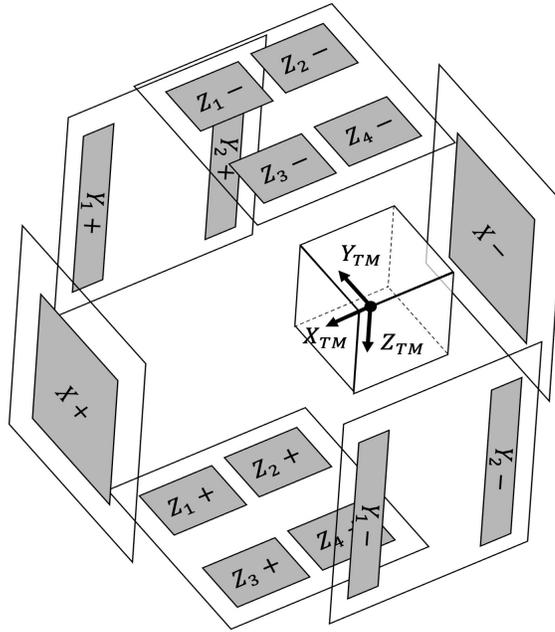
**Figure 1. S-GRS's Test Mass with Sensing and Actuation Electrodes**
