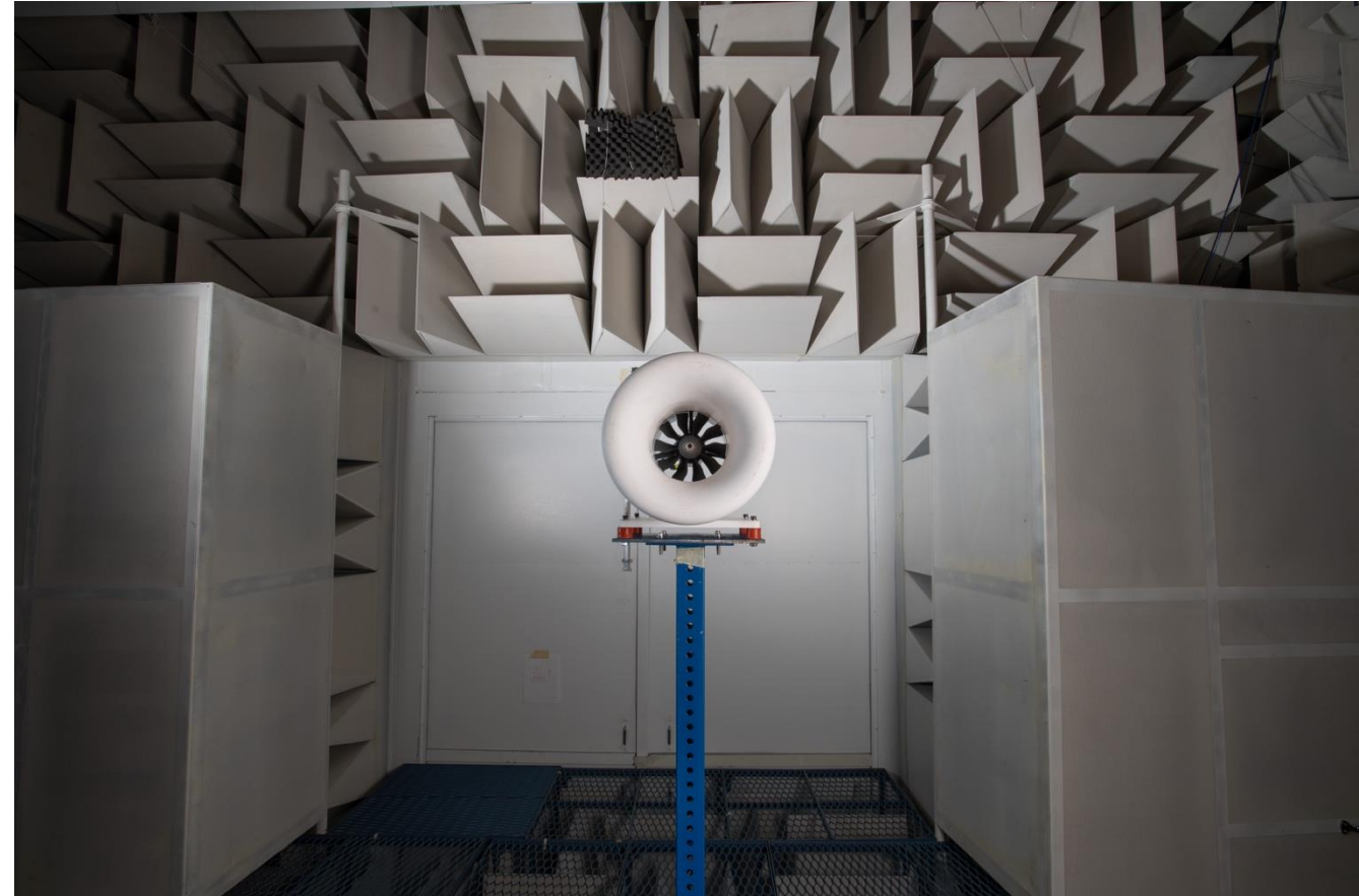
Photograph of the QUEEN V1 test set-up in the NASA GRC Acoustical Testing Laboratory, forward looking aft.
