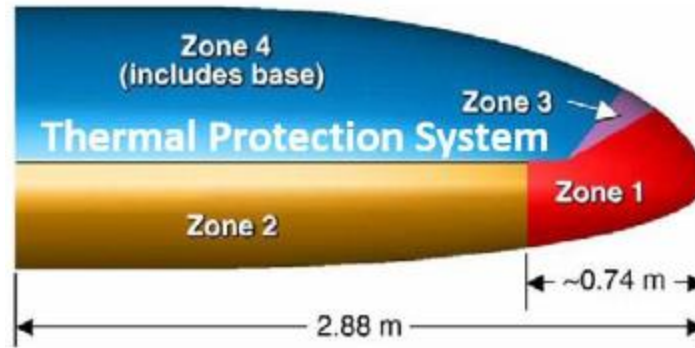
Figure 16. Vehicle Details for a Mid-Lift-to-Drag Ratio Concept (Courtesy of Lockwood, 2004) 41 .
