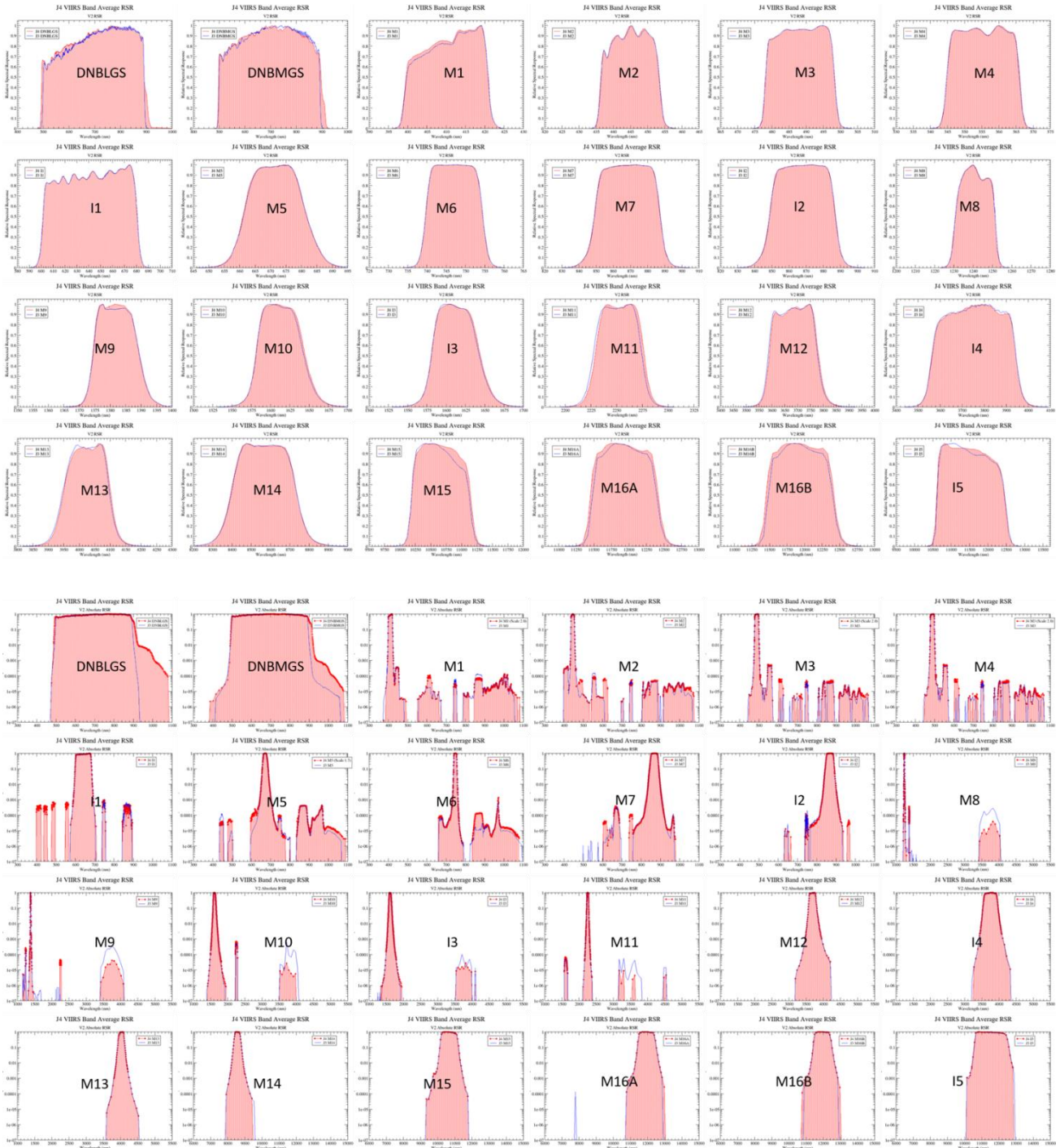
Figure 5. JPSS-4 VIIRS V2 RSR highlighting in-band (top section) and out-of-band region (lower section) for all bands measured during the pre-launch test program. Very close spectral agreement is seen between the JPSS-4 (red shaded) and JPSS-3 RSR (blue) for the in-band region (top section) with only minor differences in shape in a few bands. Out-of-band response is also very similar in JPSS-4 and JPSS-3 with some exceptions, e.g. a decrease in the 3500-4000 nm feature in bands M8, M9, M10, I3, and M11.
