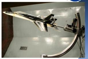
**Model mounted on C-Strut**
