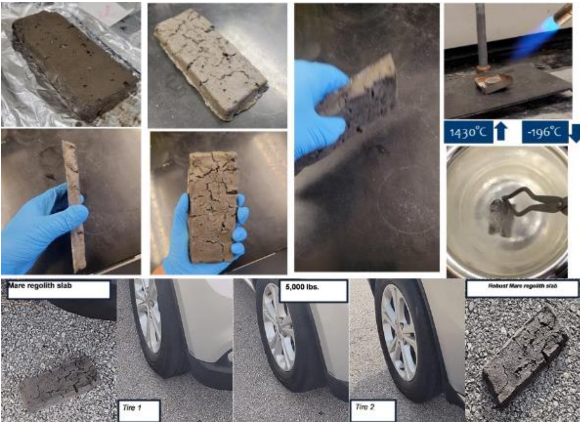
Figure 34. “Taming Regolith”: Bricks of Lunar Mare regolith constructed using silicate condensation chemistry. The bricks survive repeated impact on a stone surface as well as large extremes of temperature ranging from -196 to 1450°C and the bottom pannel shows that the bricks can sustain >5000lbs of weight.
