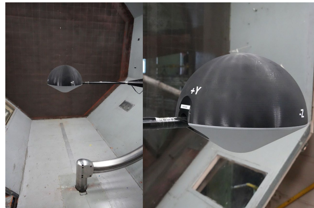
Forced oscillation test set up
