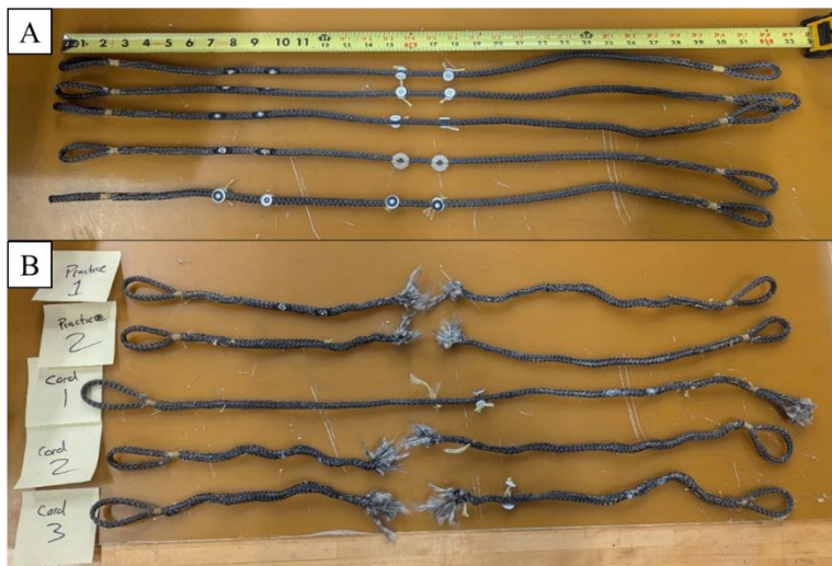
Fig. 6 Cordage Tensile Specimens A) Pre-Test With Marker Targets and B) Post-Test
