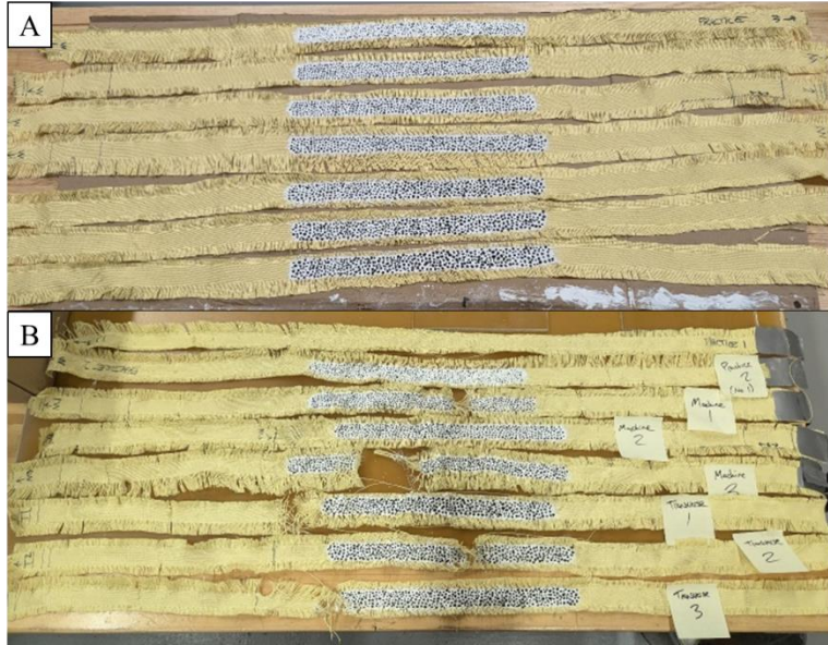
Fig. 5 Broadcloth Tensile Specimens A) Pre-Test with Speckle Pattern and B) Post-Test
