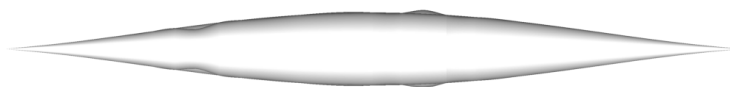
Fig. 19. Bump/divot design variables modeled on axisymmetric body as compared to baseline (vertical scaled by 2).
