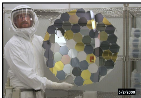
Fig. 2 Bulk collector array after mounting collectors.
