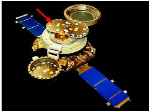
Fig. 1 One of 3 solar wind regime collector arrays unshaded in solar wind capture configuration (red arrow).
