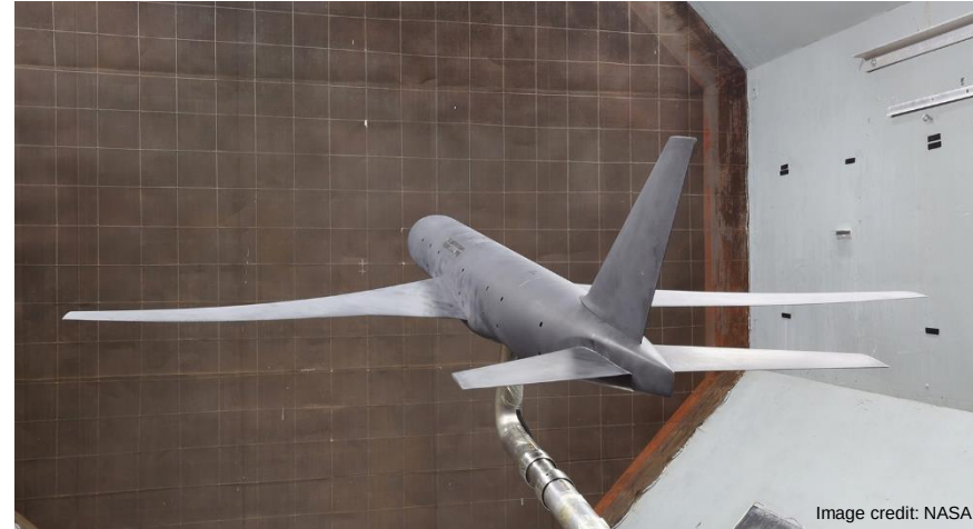
Common Research Model in the NASA Langley 12-Foot Low-Speed Tunnel.
