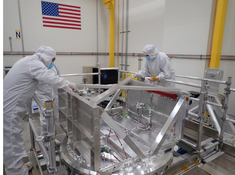
NASA/JPL-Caltech Europa Clipper Vault 9.2mm (362mil) Al-7075 ~1.4mx1.4mx1m, 150kg estimate
