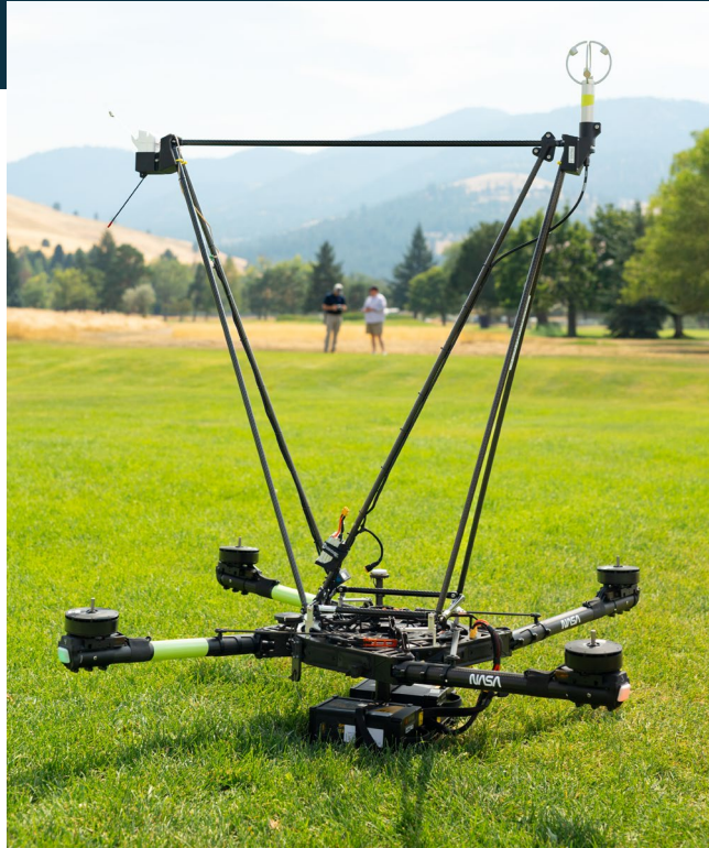
NASA Alta X vertical sounding data collection in a smoke impacted environment. NASA ARC/Milan Loiacono
