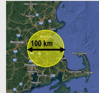
Radio Frequency Ka Band (26 GHz) 4.9m Antenna → 100 km Spot
