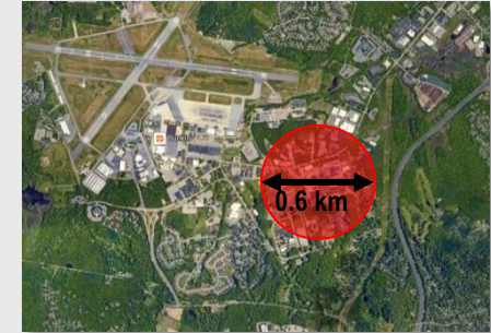
Optical C-Band (1550 nm) 10-cm Antenna → 0.6 km Spot
