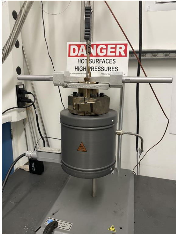
Figure 2. Image of the small Venus In-Situ Chamber (Lil'VICI) at NASA Goddard [10].
