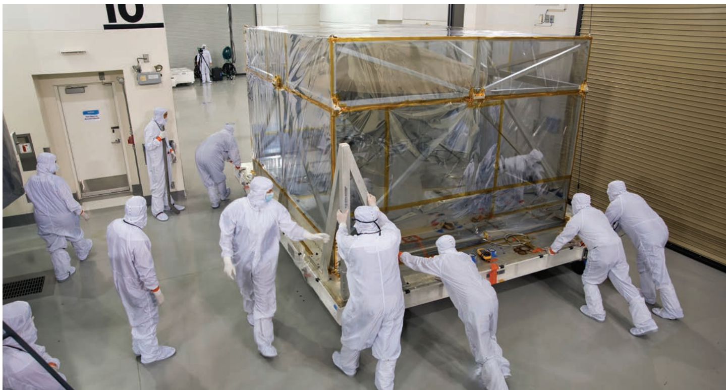
Figure 26: Inside the Astrotech processing facility at Vandenberg Air Force Base, the InSight spacecraft was removed from its shipping container and positioned for removal of protective wrapping. Photo credit: NASA
