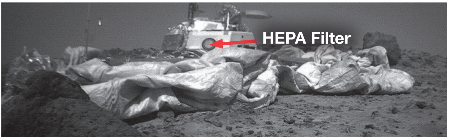
Figure 31: Mars Pathfinder photo on Mars taken by Sojourner camera, showing the integrated subsystem assembly (ISA) HEPA filter. Photo credit: NASA
