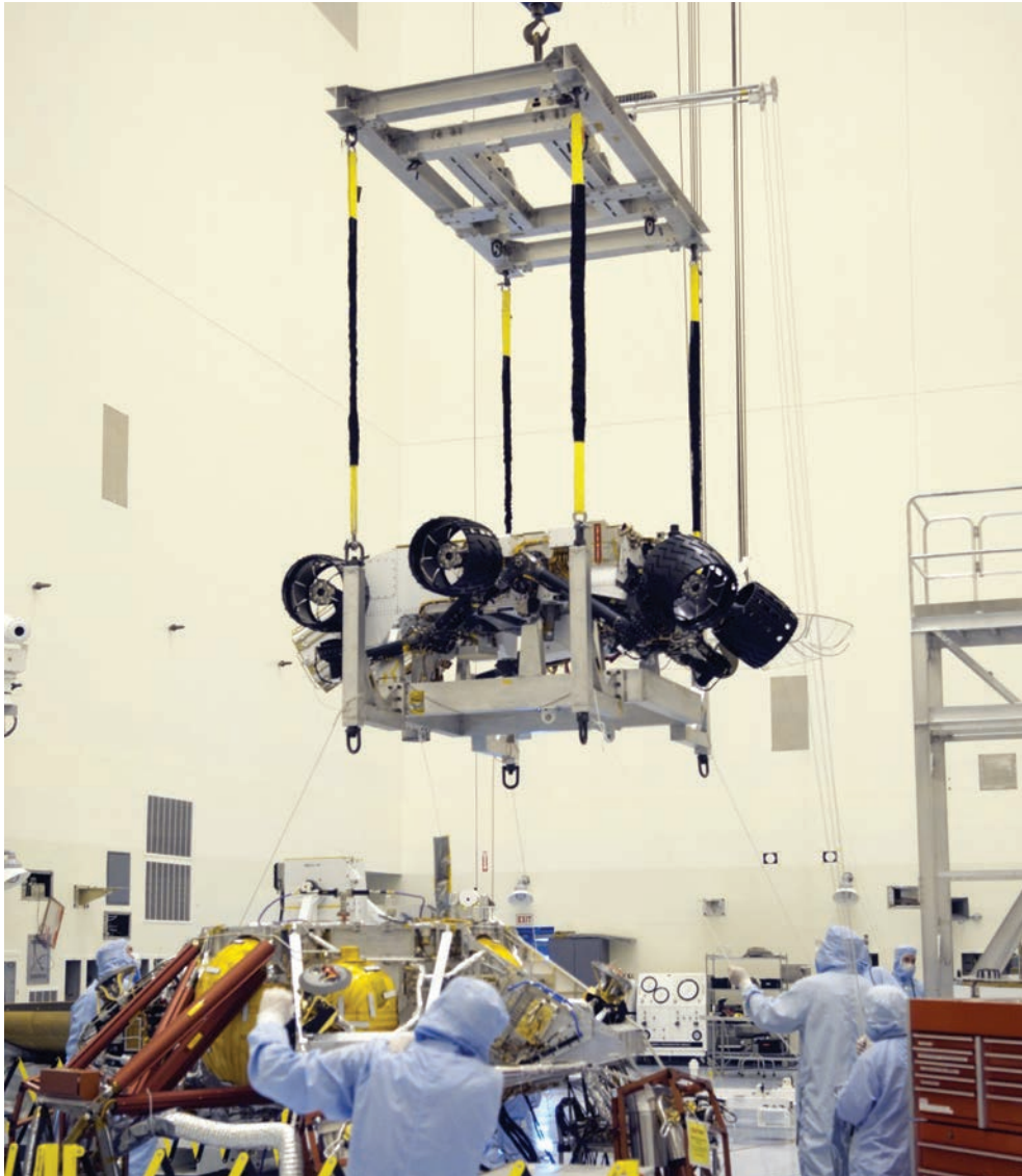
Figure 24: Technicians using an overhead crane in the Payload Hazardous Servicing Facility at Kennedy Space Center lift the Mars Science Laboratory (MSL) rover, known as Curiosity, for its move to a rotation fixture for testing. Photo credit: NASA
