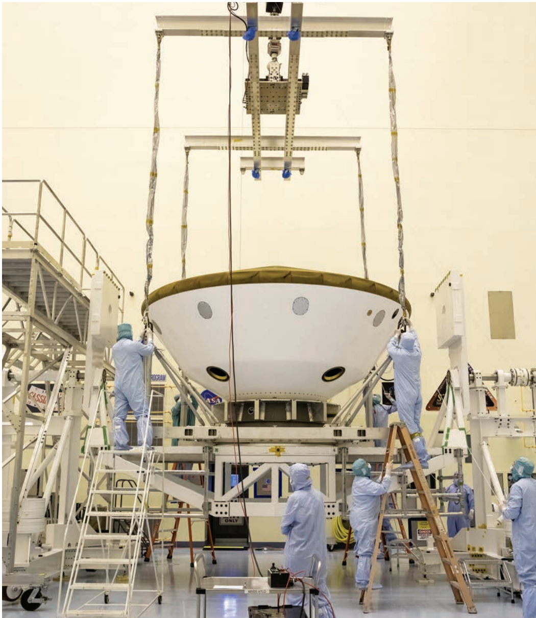
Figure 27: Mars 2020 Lift Activities in Payload Hazardous Servicing Facility (PHSF) Photo credit: NASA
