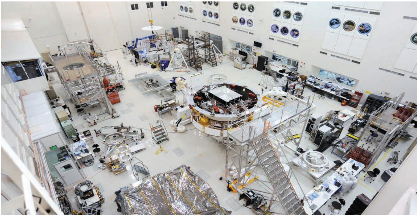
Figure 21: This image shows major components of NASA's Mars 2020 Mission in the High Bay 1 cleanroom in the Jet Propulsion Laboratory's (JPL's) Spacecraft Assembly Facility. The spacecraft is in the center of the photo. Note all of the GSE in the area to support assembly activities. Photo credit: NASA
