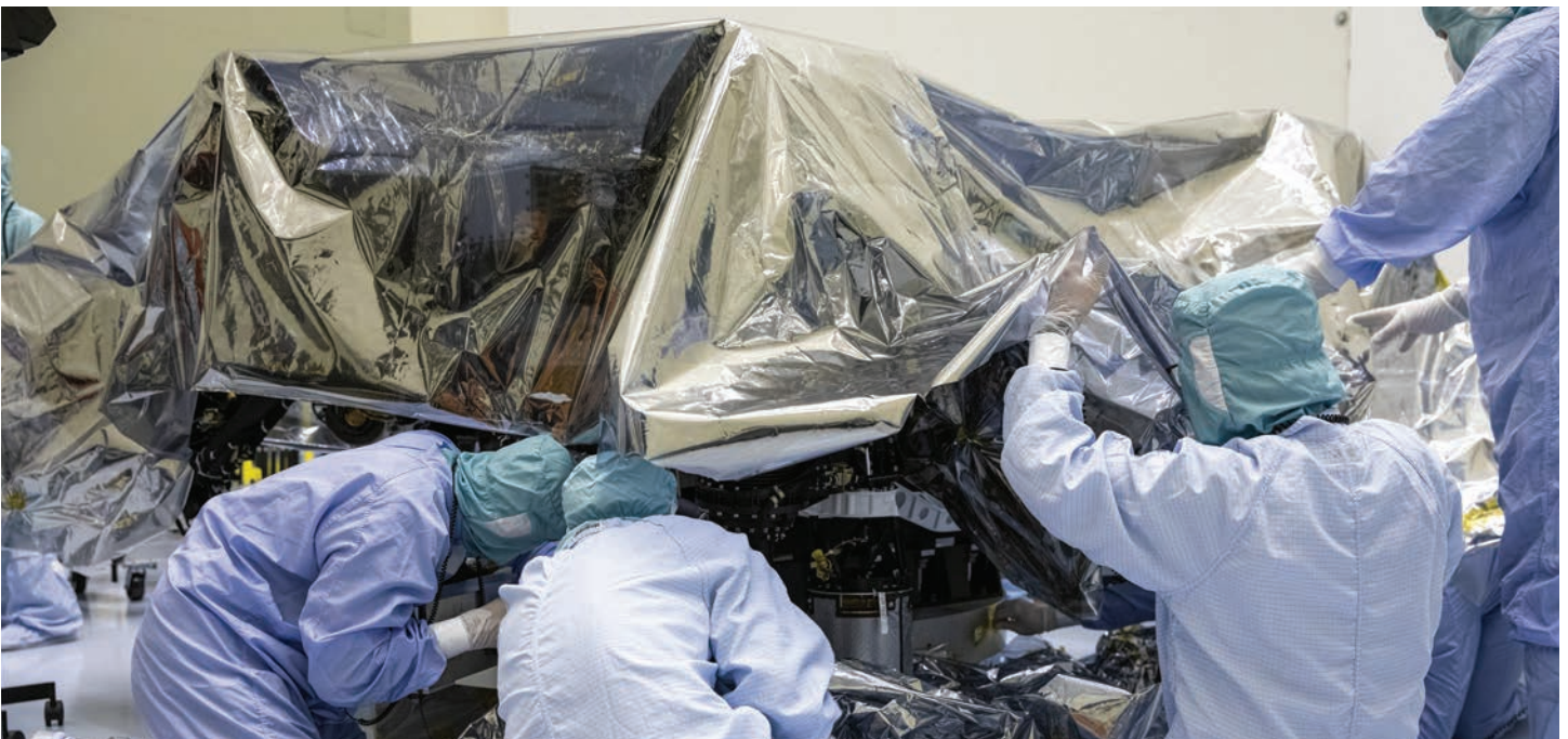
Figure 29: The Mars 2020 rover undergoes processing inside the Payload Hazardous Servicing Facility at Kennedy Space Center. Note the rover is covered to prevent environmental cross-contamination. Photo credit: NASA
