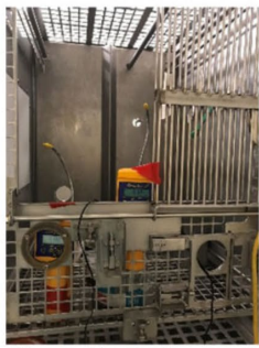
Figure 1b: Portasens II - Parametric testing of O 3 and H 2 O 2 concentrations during decontamination.
