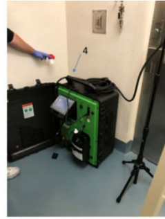
Figure 1d: Sample 4 located behind the iHP application nozzle. Also, view decontamination equipment.
