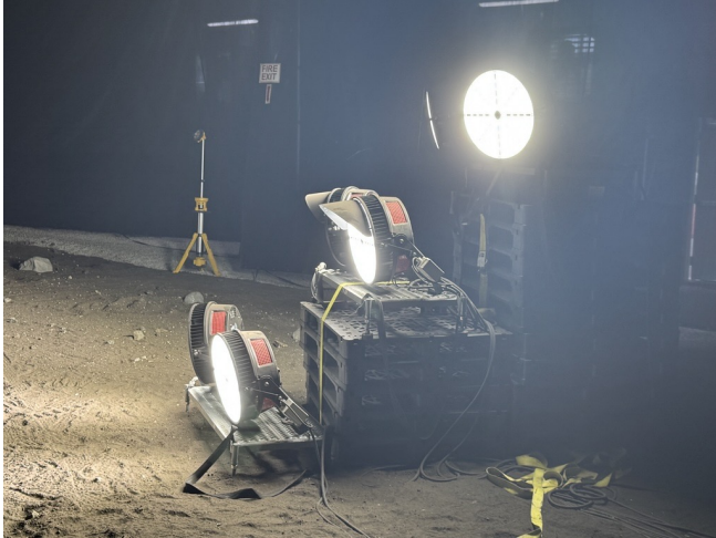
Figure 9: The six RuggedGrade StadiumPro IV 1400W lights used as solar simulators in the test-site.
