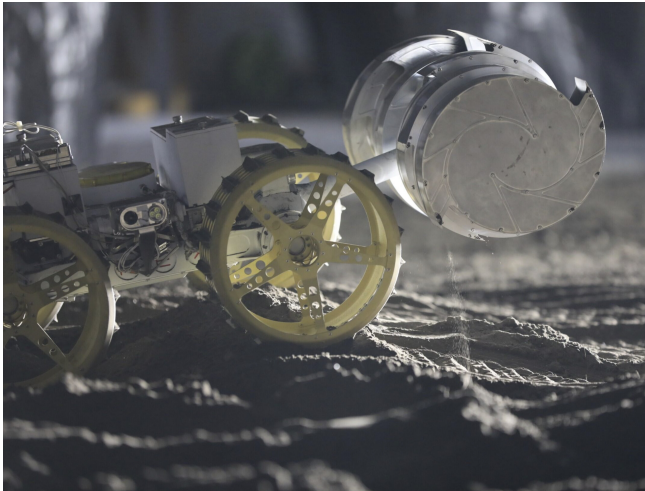
Figure 16: IPEX unloading at the ‘dump’ site. Note trail of granular material exiting bucket drum scoops.
