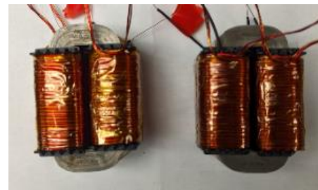
Transformer prototype (110 V to 3,000 V)
