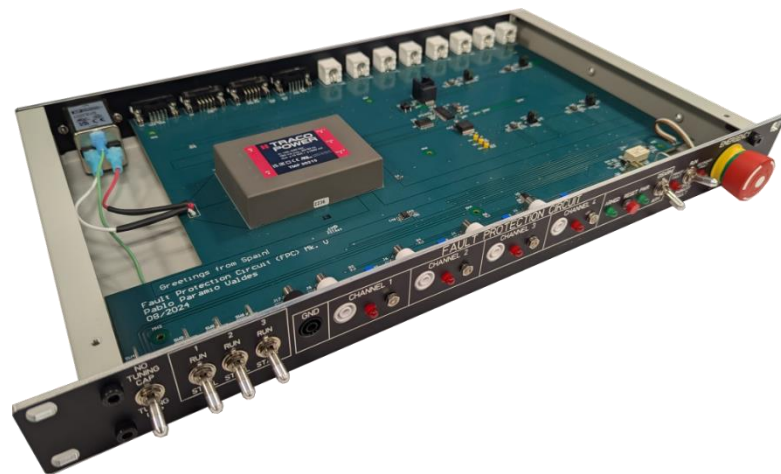
Fault Protection Circuit front and rear
