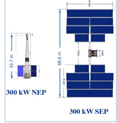
Nuclear Electric Propulsion (NEP) heat dissipation panels as compared to Solar Electric Propulsion (SEP)<sup>4</sup> solar panels.
